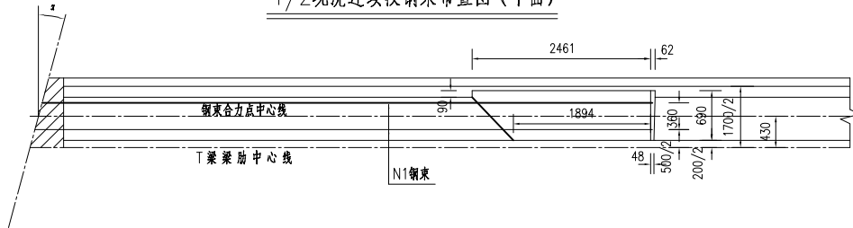
1/2现浇连续段钢束布置图(平面)
